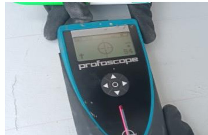
REBAR SCANING TEST
